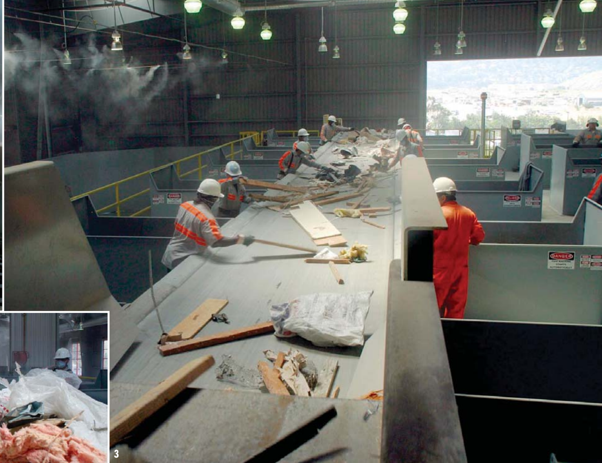
1) All unprocessed material is initially screened to remove fines. 2) Sorters pull out paper, unpainted wood, ferrous and nonferrous metal, unpainted sheetrock, cement, brick, green waste, cans and bottles. 3) Recovered materials (e.g. wood) are dropped into bunkers under the sorting line.
